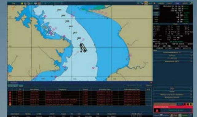
Each Alert is separated into 3 grades, ALARM (Red) / WARNING (Orange) and CAUTION (Yellow), and are displayed in the order of priority.
