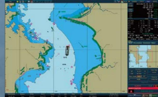
Selected Route route check (dangerous objects/collision avoidance), route monitoring (Off Track, Grounding avoidance) and Own Ship's Guard Frame display dangerous information (With regards to the conditions set)
